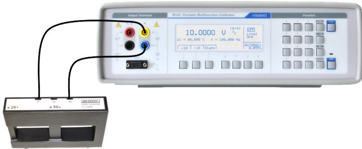
Figure 7 Current coil connection
